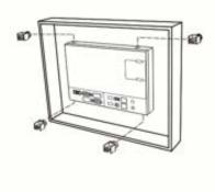
Step 4: For heat dissipation, please keep a minimum clearance of 60 mm on the rear of the HMI.
